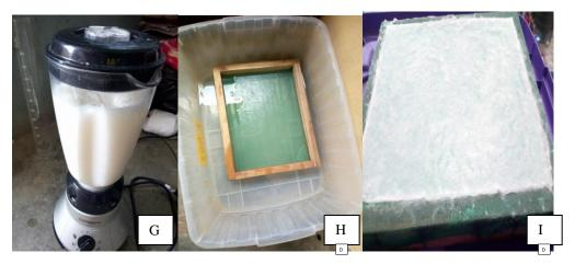
Figure 4: Sheet making process; G = Pulp blending, H = pulp pouring, I = Sheet draining
