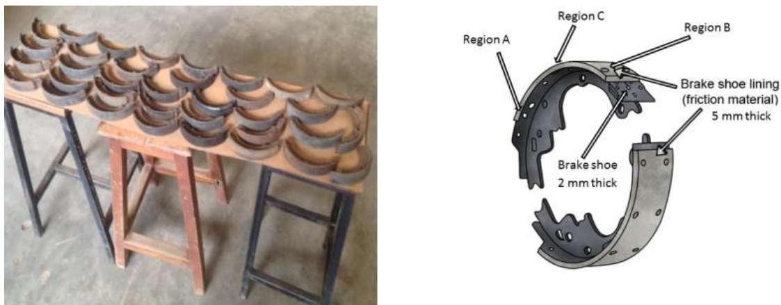
Figure 1 Tricycle brake lining; (a) collected 30 samples, (b) measured height of worn regions
