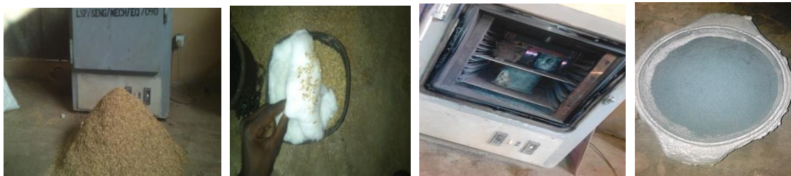
Plate 2: (a) Rice Husk (b) Rice husk lagged with cotton wool (c) Furnace for Carbonating the rice husk (d) 150 µm Rice Husk Ash
