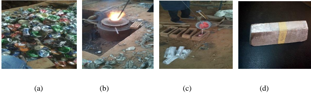
Plate 3: (a) Aluminium Scrap (Waste Aluminium Can) (b) Aluminium scrap melting in crucible furnace (c) Pouring of molten metal and Aluminium alloy billet (d) Control Sample
