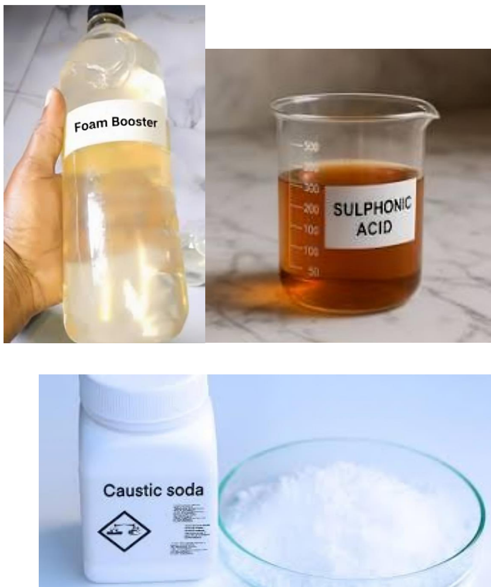
Fig 2: A, B, C & D Showing Foam Booster, Sulphonic Acid (Labsa), Caustic Soda, And Nitrosol Used in Liquid Detergent Production
