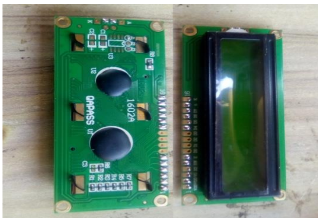
Figure 6: Front and back view of the LCD
