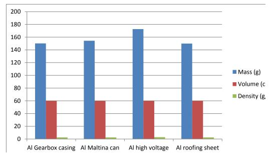
Fig 5: Chart of the mass, volume and density of the aluminium bars
