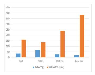
Fig.8: Results of impact and hardness of the materials
