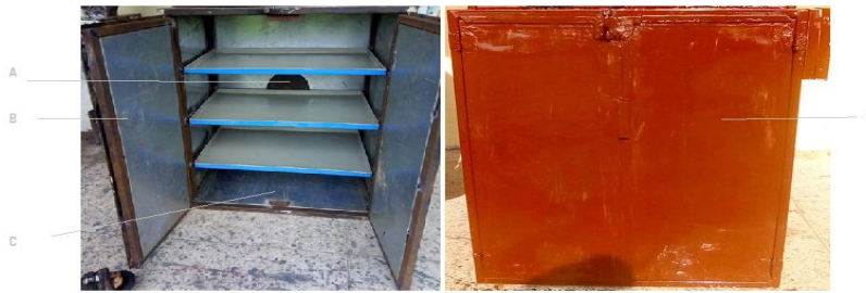
Keys: A- Electric heating element; B-Door; C—Position for charcoal tray; D Oven door
