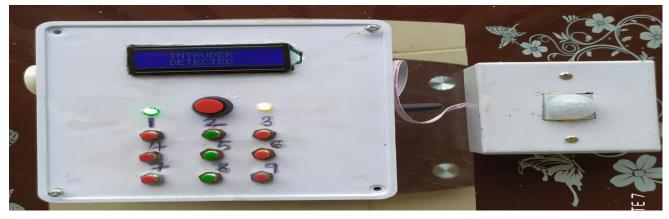
Figure11.0 (a): Intruder detected by the system
