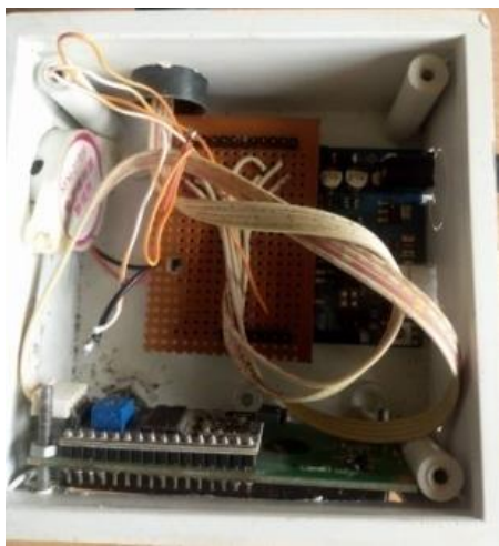
Figure 3: Internal Packaging of the circuit board
