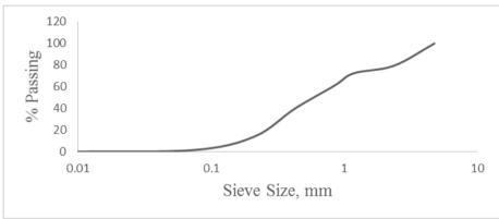
Figure 1: Particle size distribution
