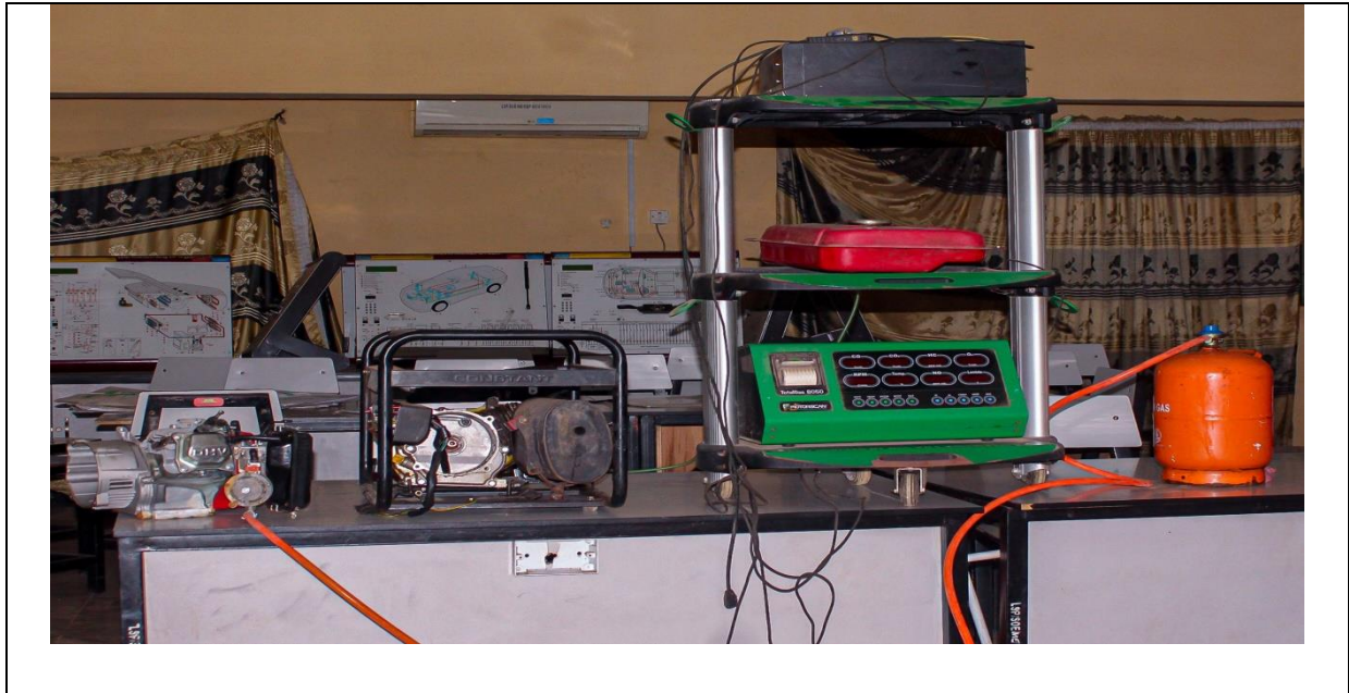
Figure 4 Set-up of the experiment after conversion of a gasoline generator to CNG fuel
