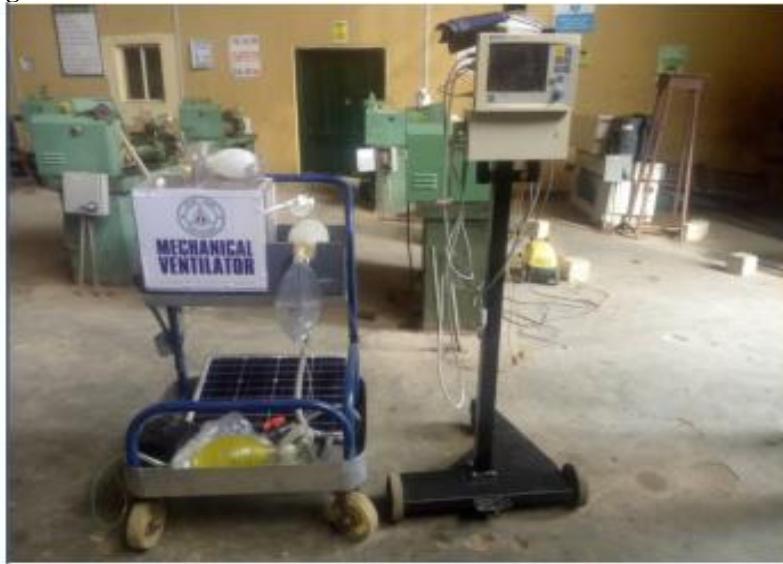
Figure 9 : Completed mechanical ventilator unit with a monitor and solar panels
