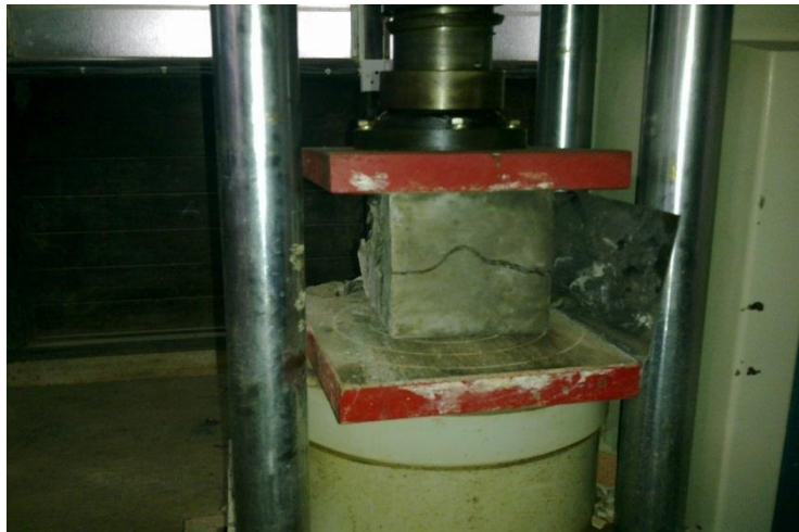
Figure 2: Concrete cube under compressive failure
