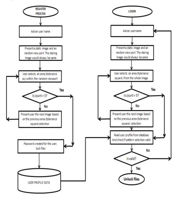
Fig. 6. Data Flow diagram
